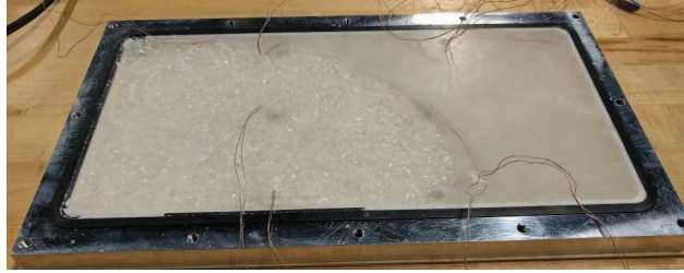
Figure 3.6.: PCM test setup with thermocouples embedded in the plate.
