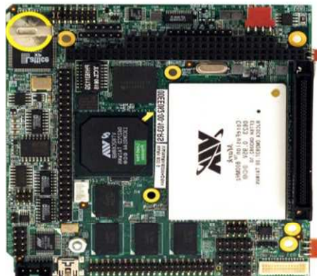
Figure 8.3: Athena II SBC by Diamond Systems®.
