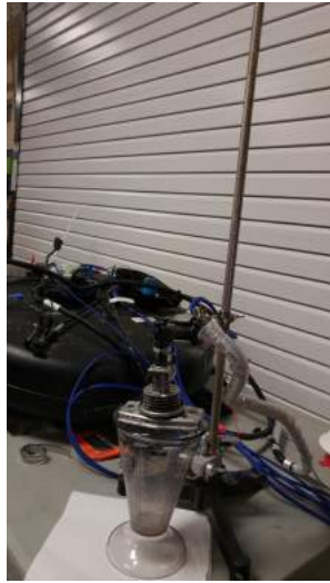
Figure 4.6.: Injector Calibration Setup and off, it is easy to control the injector duty cycle by varying the PWM signal duty cycle. Table 4.1 below shows the results from calibration.
