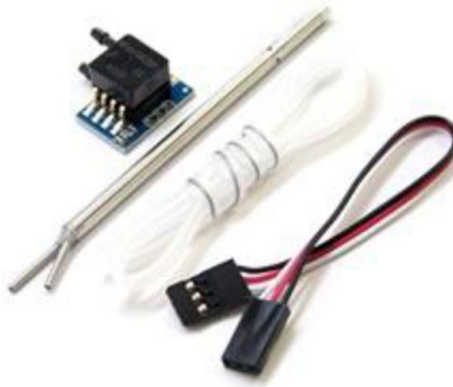
Figure 24: Airspeed Kit with the MPXV7002DP differential pressure sensor by Freescale Semiconductor.
