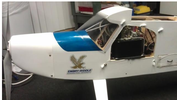
Figure 10: Sig Rascal 110 with the primary flight computer installed.
