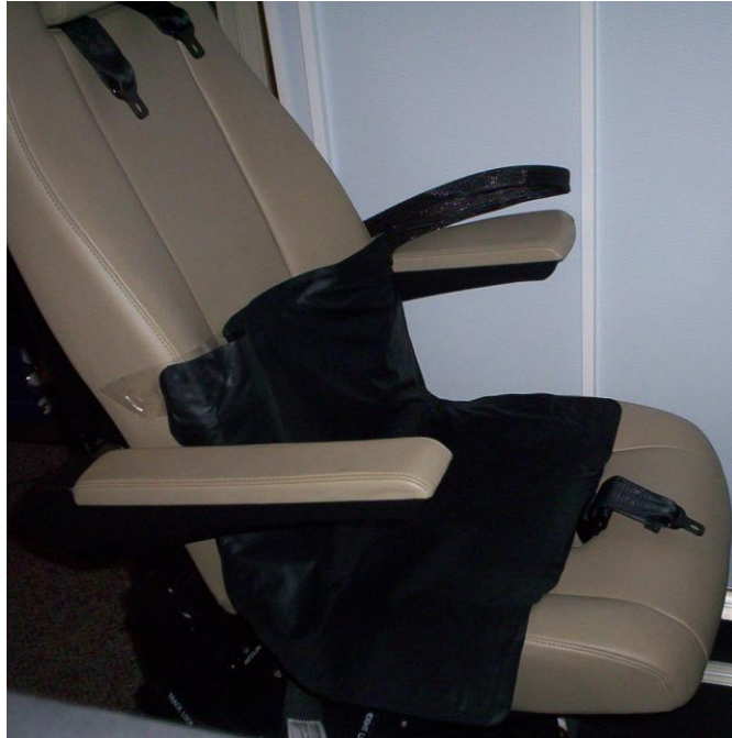
Figure 7. Example of pressure pad placements.
