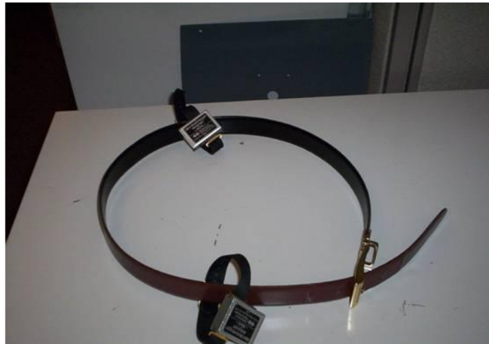
Figure 9. Actigraph belt. Participants placed the belt around their waist during the time he or she sat on each seat.
