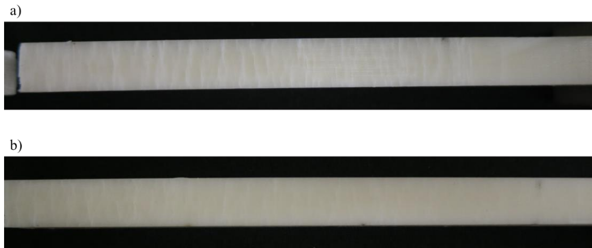
Figure 3.4 Close-up image of crazing in a) ASTM D638 and b) ASTM D3039
