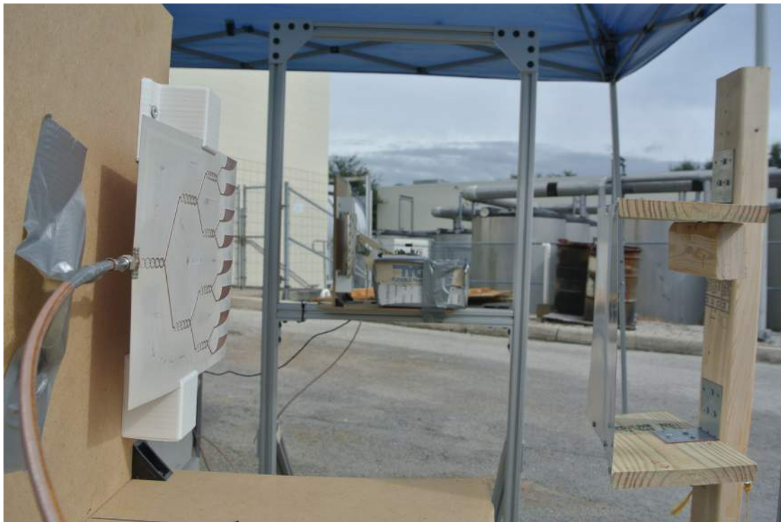
FIGURE 3.37: Elliptical RF reflector during testing
