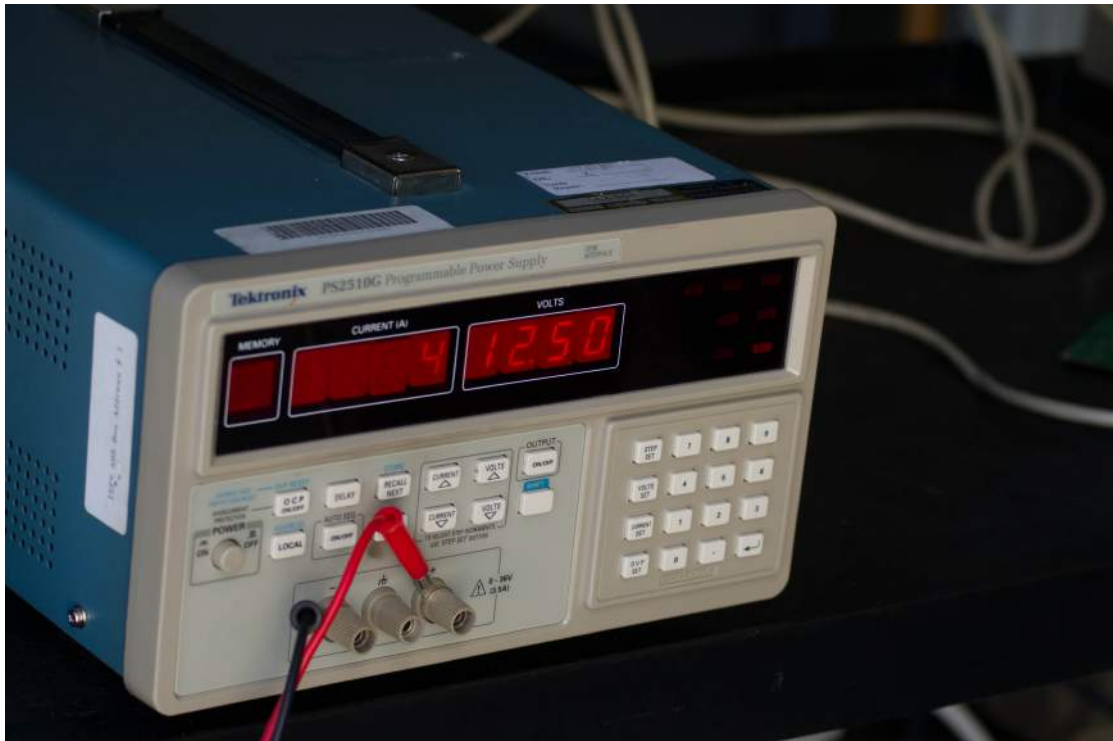
FIGURE 3.24: One of the set of three DC power supplies
