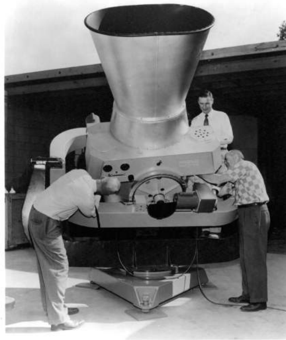
Figure 1.2: The Baker Nunn camera for satellite tracking with Joseph Nunn and manufacturers Clyde Chivens and Harry Boller. FROM BOLLER AND CHIVENS [2011].
