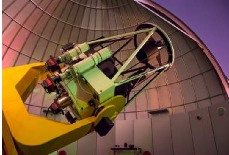
Figure 4.10: The DFM 1 m telescope at Embry-Riddle's Daytona Beach campus. With over 8 m of focal length, the field of view is very small with most detectors. Several telescopes are co-aligned with the main telescope to provide a variety of fields of view. FROM observatory.db.erau.edu , COPYRIGHT MICHELLE BLAKE.
