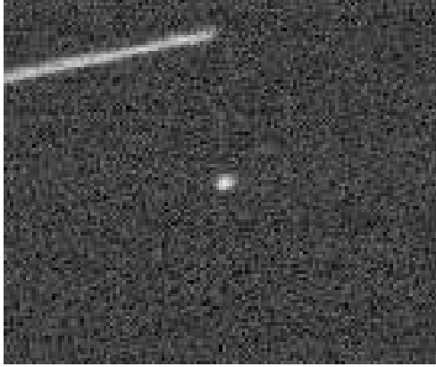
Figure 3.3: A cropped, unfiltered .fits image of the POPACS-2 nanosatellite acquired January 20, 2016 at 10:46:17.895 UTC using OSCOM’s RASA telescope in Daytona Beach, FL. The bright line in the upper left is a star streaking through the field of view as the telescope tracks the satellite.
