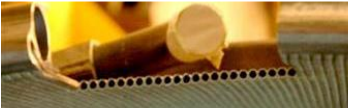
Figure 2: Regenerative Cooling Channel Cross Section [21].
