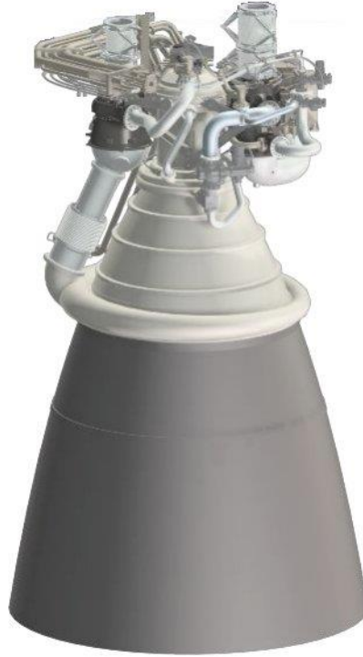
Figure 3: Computer model of the J2-X SSFC engine currently under development [31].
