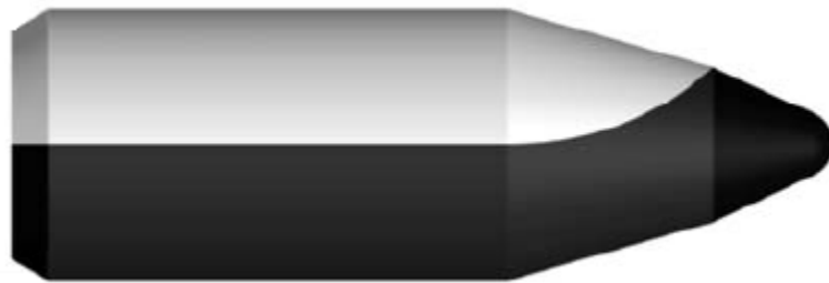
Figure 7 – The Mars multi-use shroud option is comprised of a thickened composite sandwich material to provide micro-meteorite protection and an ablative thermal protection surface [49] . Utilization of composite materials will also minimize overall mass, thus, propellant requirements for the launch vehicle. The TPS (illustrated as black in the figure) provides thermal loading protection during entry and descent en route to deploying that mission payload to the Martian surface.
