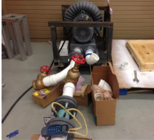
Figure 3-11: Experimental blower used with control valves.
