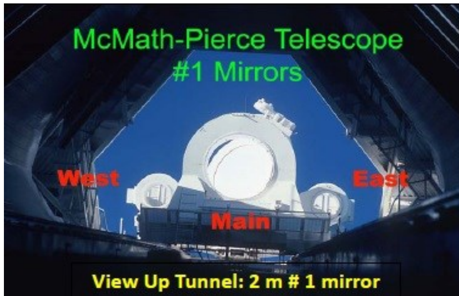
Figure 2.2: View of the #1 mirrors for the Main, the East auxiliary, and West auxiliary as seen from inside the telescope, viewing straight up the tunnel. The cover for the #1 mirror is open while the #1 mirror covers are closed for both auxiliary telescopes.
