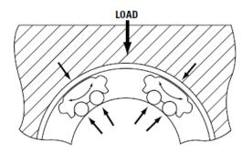
Figure 3.23: Close-up of Double Track Bearings Showing How They Self-Align (roll) to Evenly Distribute the Load on Each of Their Two Ball Tracks [23]
