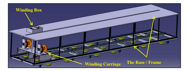
Figure 3.1: Showing Assemblies, Sub-Assemblies of the Compliant Winder Machine, CWM \*Note that the control box is not shown since this thesis will not be covering the details
