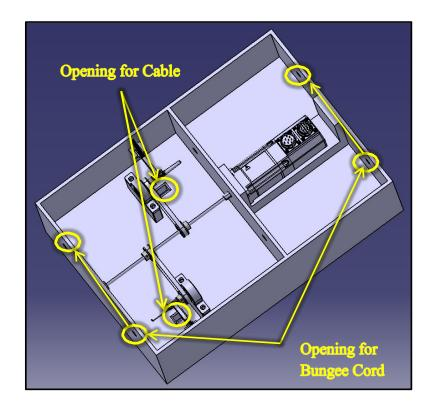
Figure 3.29: Inside of the Winding Box Shown
