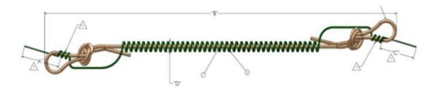
Figure 1.1: Compliant Wind Concept Shown with the Bungee (Rubber) Passing Through the (Green) Wound Compliant Cable
