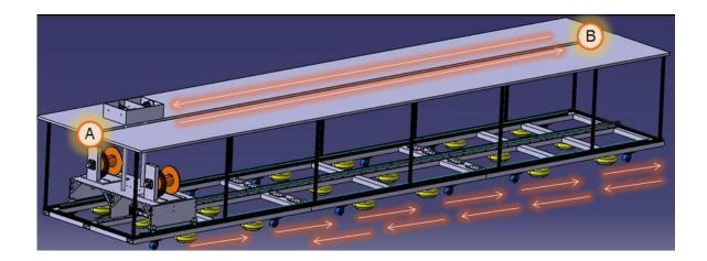
Figure 3.30: The Final Design of the Compliant Wind Machine Shown with A Representing the Initial Position and B Presenting the End Position
