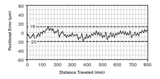
Figure 3.15: Regardless of the Distance Traveled, Positional Accuracy Remains Constant With the RPS System [22]
