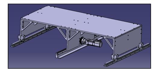
*Figure 3.12: Isometric View of the Base Structure with the Emerson NTE-212-CONS-0000 Servo Motor and an APEX Gear Reducer on the Winding Carriage*
