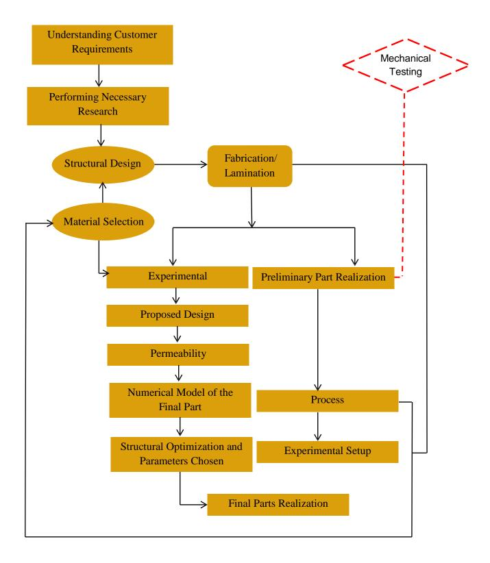
Figure 2.4: A Flowchart Representing the Design Process for Machine Design [3]
