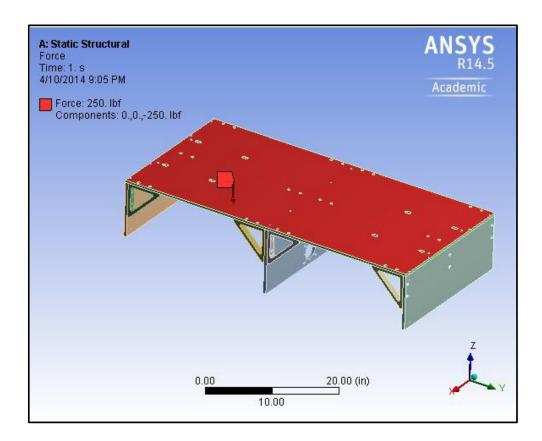
Figure 4.3: Model of the Wind Carriage Shown With Applied Load
