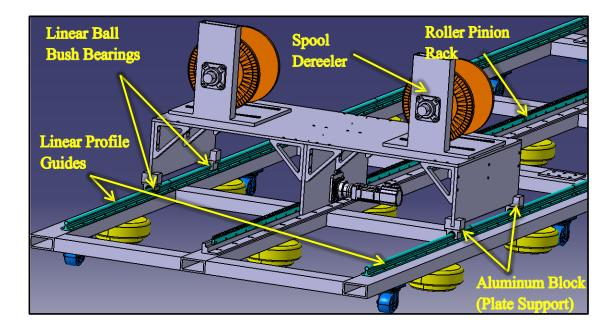
Figure 3.3: Isometric View of the Base Structure with the Linear Guide System of the Winding Carriage
