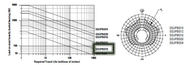
Figure 3.24: Available Super Smart Ball Bushing Pillow Blocks Sizes for Continuously Supported Applications (Top); Load/Life and Polar Graph with Lines Indicating Limiting Load for Given Ball Bushing Bearing (Bottom) [23]
