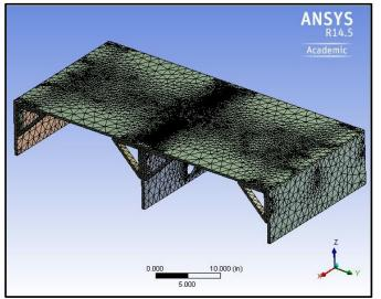
Figure 4.2: Model of the Wind Carriage Shown With 0.10 Mesh Applied in ANSYS
