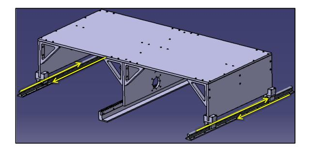
*Figure 3.2: Isometric View of the Base Structure of the Winding Carriage Shown Without the Spool and Spool Dereelers on Top; The arrows indicate the linear motion it performs.*
