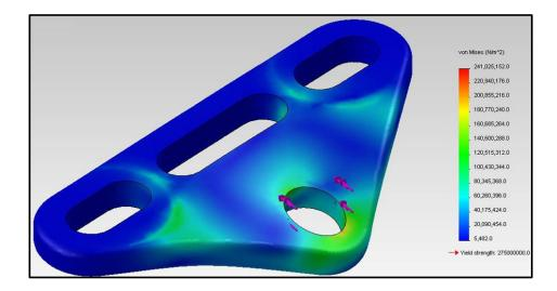
Figure 2.3: Results of a Finite Element Analysis Study on a Plate Showing the Maximum Stress and Deformation [7]
