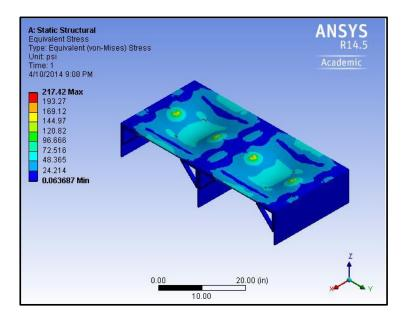
Figure 4.4: FEA of the Wind Carriage with the Von Mises Stress Shown
