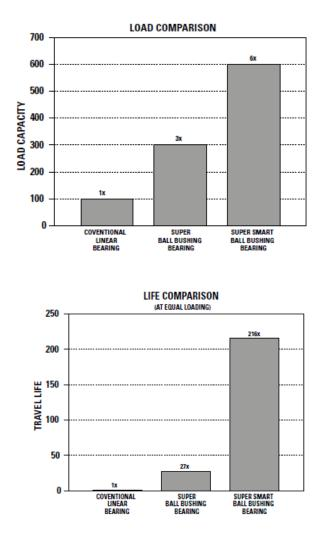
Figure 3.25: Comparing the Load and Travel Life between the Conventional, Standard and Super Smart Ball Bushing Bearings [23]
