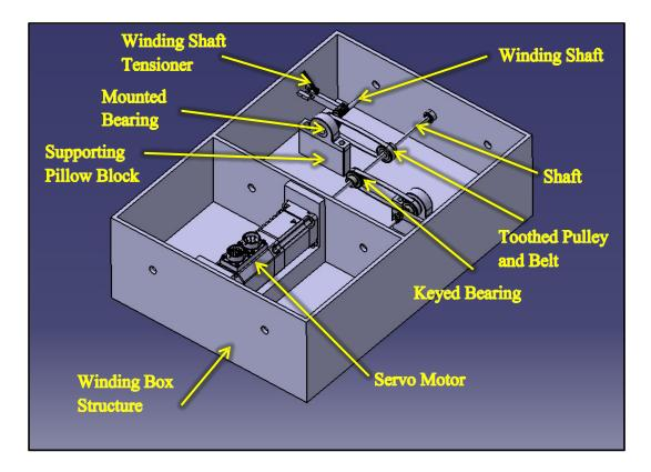
Figure 3.28: Components of the Winding Box Shown
