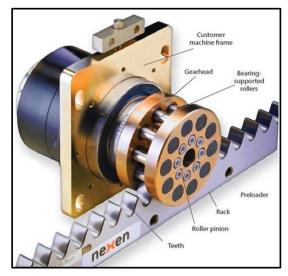
Figure 3.14: A Roller-Pinion System, RPS with Its Components Shown from Nexen Group Used in the New Compliant Wind Machine [22]
