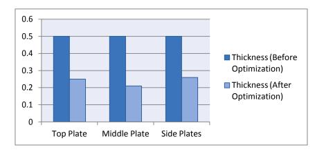
Figure 4.7: The Comparison of Thickness Extracted from HEEDS for the Top, Middle and Side Plates of the Carriage
