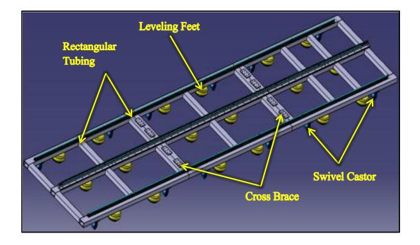
Figure 3.26: The Base of the Compliant Wind Machine shown With Leveling feet and Castors
