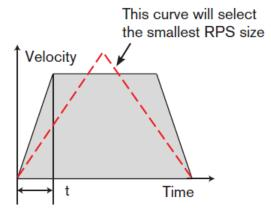
Figure 3.17: Acceleration Based on Time (t) [22]
