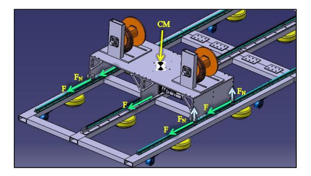
Figure 3.9: Applied Loads and Acting Forces Shown on the Wind Carriage, where F = Horizontal Force, FN = Normal Force and CM = Center of Mass
