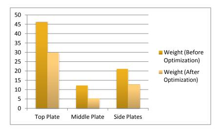
Figure 4.8: The Comparison of Mass Extracted from HEEDS for the Top, Middle and Side Plates of the Carriage
