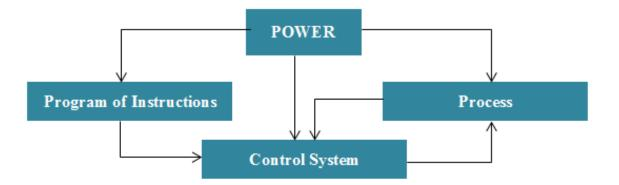
Figure 2.2: Basic Elements of an Automated Machine (Power, Program of Instructions, Control System) Resulting to the Final Process [6]
