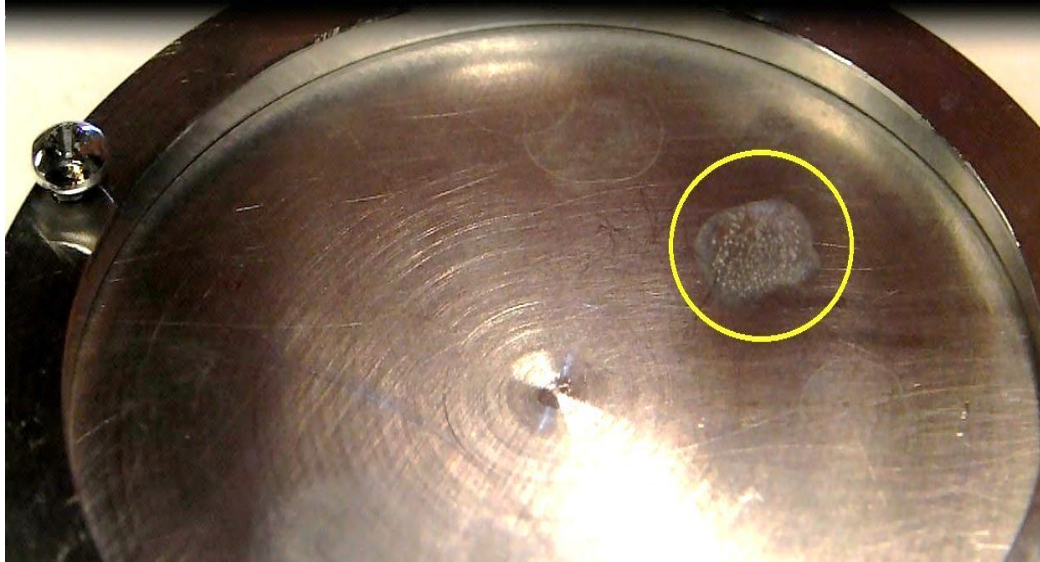
Figure 3.30: Nucleate boiling regime
