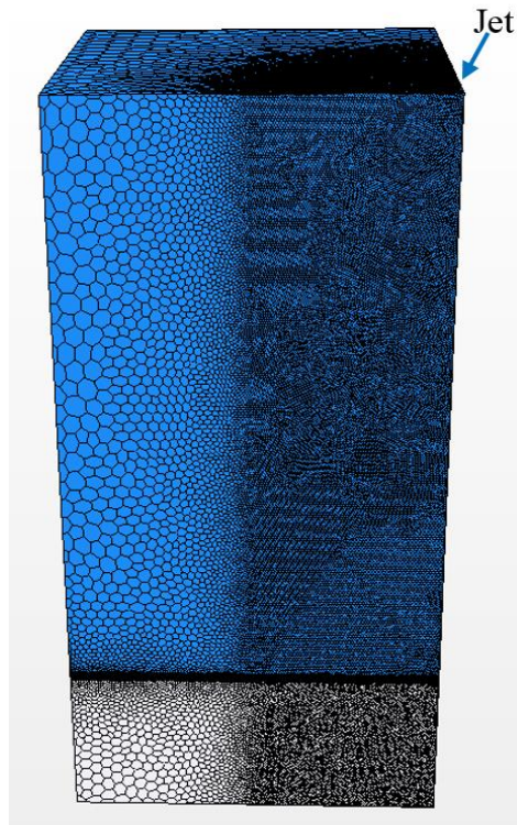
Figure 5.4: Mesh Model of a Quarter Impinging Jet for a Rocket Nozzle Throat Cooling Geometry
