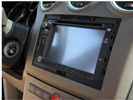
Figure 37: IDEA Computer with Student Designed Bezel
