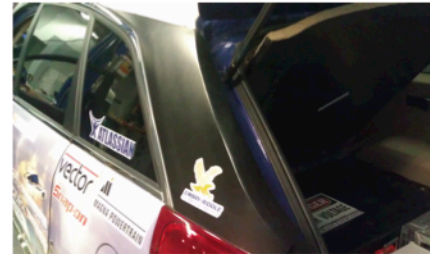
Figure 8: D-Pillar Aerodynamic Modification
