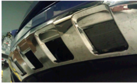
Figure 6: Bumper Cut-Out Aerodynamic Modification
