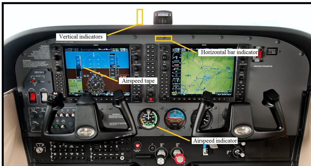
Figure 5. Location of the AOA indicators in relation to the airspeed tape on the G1000 and standalone airspeed indicator.
