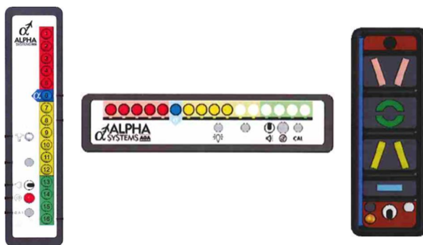
Figure 2. The three AOA indicators preselected by the flight department for the proposed study. vertical bar, horizontal, bar, and legacy indicators.
