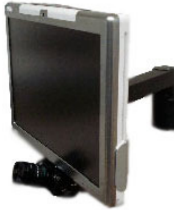
Figure 1: An example of a fixed eye tracking system mounted to a computer monitor (LC Technologies, 2009).
