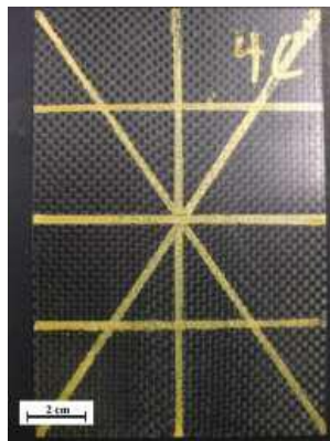
Figure 13: 4 by 6 in. laminated graphite/epoxy coupon [1]
