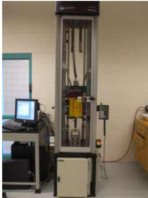
Figure 14: Instron Dynatup 9200 calibrated impactor [1]
