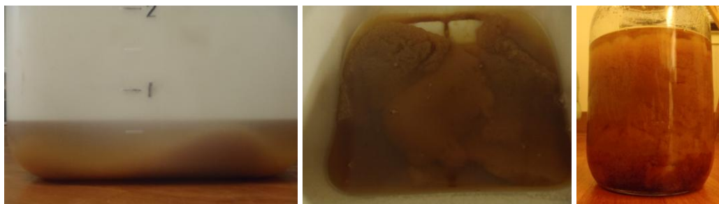
Figure 15. Results from the third test batch. In the third test batch, the biodiesel did not properly react and formed into a combination of a liquid and a jelly-like substance. The image on the left shows how the mixture looked from the outside of the mixing container. The center image is taken from the top of the mixing container, and the image on the right shows what the mixture looked like when poured into a clear glass jar.
