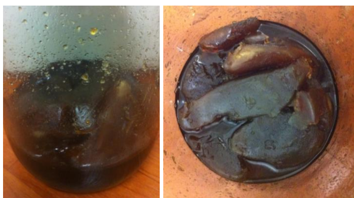
Figure 13. Chunks of 'gunk' after sitting in sun. These images indicate how the chunks of 'gunk' transformed into soap from sitting out in the sun for a week.
