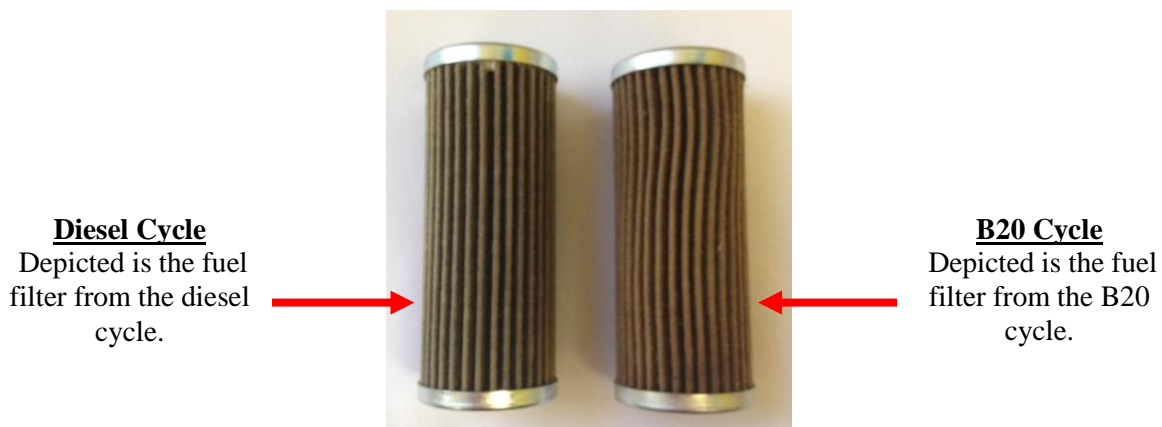
Figure 29. Fuel filter comparison of the diesel and B20 cycle. Depicted above is the fuel filter from the diesel cycle (left of image) and from the B20 cycle (right of image).
