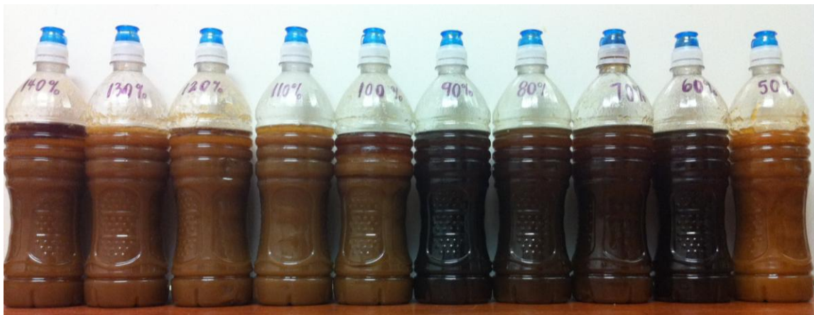
Figure 20. Results from the ten sample experiment. As the amount of catalyst increases, the ‘biodiesel’ turns into a jelly texture. As the amount of catalyst decreases, the ‘biodiesel’ turns more solid. The optimum amount of catalyst fell somewhere in between the 90% and 60% of the titration amount.
