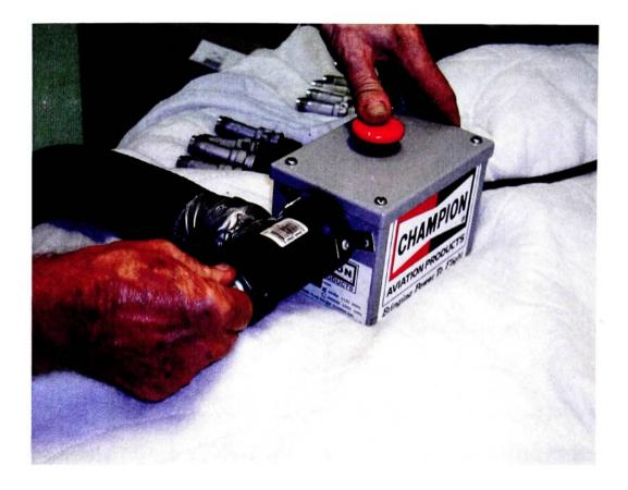
Figure 12 Local Exhaust Ventilation Control Device With User Demonstrating Spark Plug Cleaning The second recommendation is to use iridium spark plugs in place of the massive electrode spark plugs. This approach eliminates the lead exposure problem and has cost advantages described in Appendix E.
