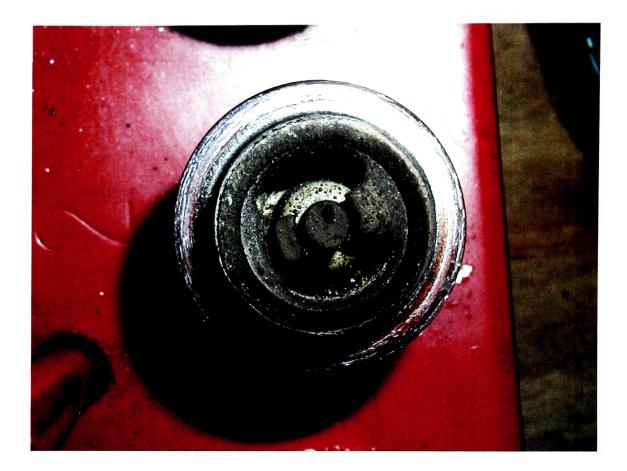
Figure 1. Spark Plug with Lead Bromide Accumulation After Fifty Hours of Time in Service
