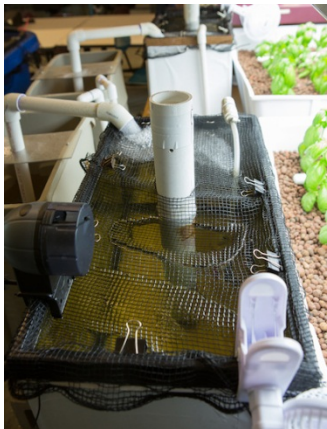
Figure 10: A picture of the fish tank. Center: The SLO casing pipe. Top left: Airlift pumping aerated water into the tank.
