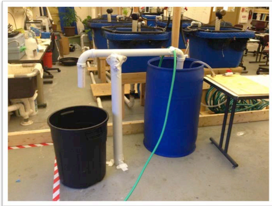
Figure B 2: A picture of the airlift experiment setup.
