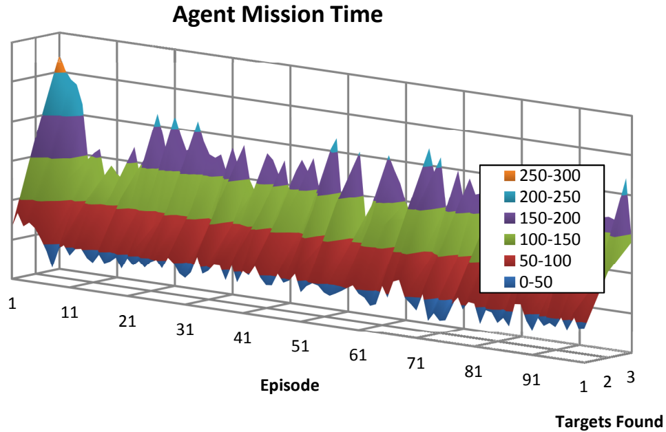
Figure 6: The Mission Time plot. A plot showing the time to mission completion for an initial reward scheme of 10 for finding a real target, -2 for an incorrect declaration, and -1 for all other outcomes. The time to locate all targets decreases for the system up to about episode 4 or 5, then it rises and attains a worse steady-state performance. The best performance was achieved when the temperature was equal to about two, indicating that the overall reward scheme should be factored by half to attain the best steady-state performance.
