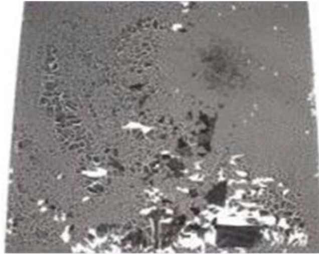
Figure 3.1 An example of micro-cracked buckypaper (Kan, 2013)
