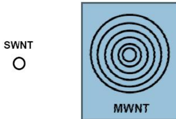
Figure 2.5 Schematic diagram of a SWNT and a MWNT (Yeh, 2007)
