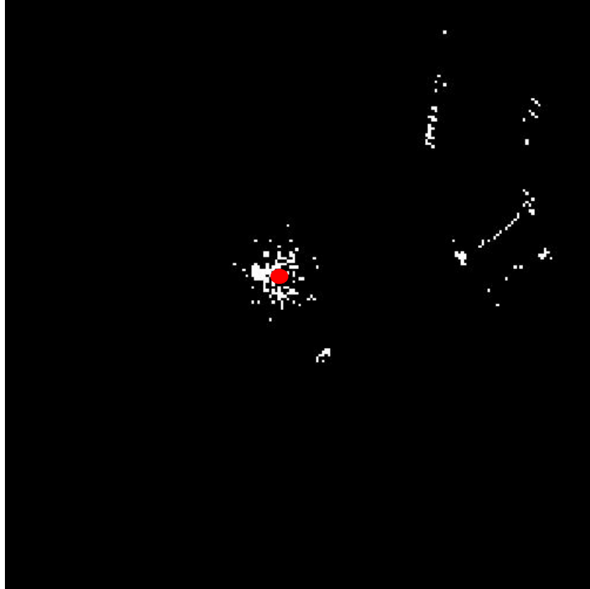
Figure 10: Initial occupancy grid showing the docks and shore on the right of the image, spurious data returns around the ASV, indicated by a red circle, and returns from the chase boat below the ASV.
