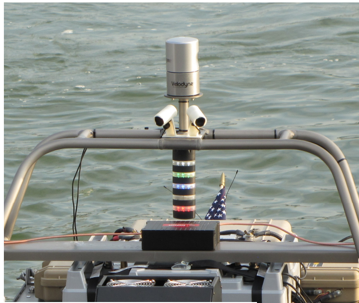
Figure 5: Minion's exteroceptive sensor suite
