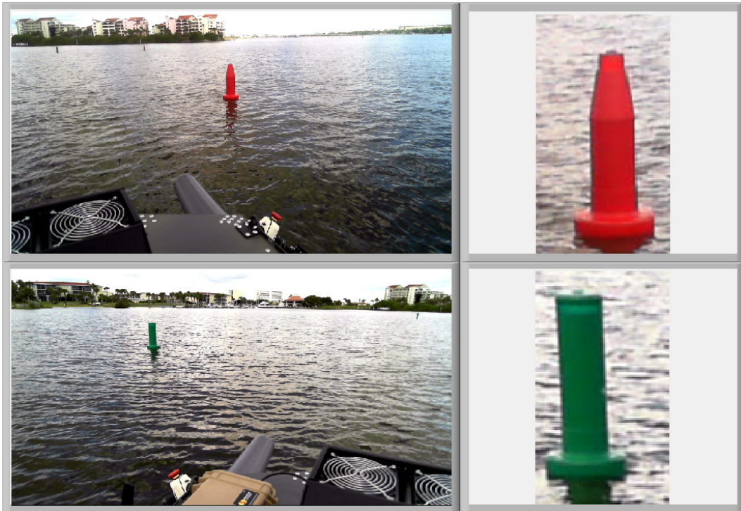
Figure 33: From top left clockwise: Right camera full image. ROI of red buoy found in the right camera. ROI of green buoy found in the left camera. Left camera raw image.
