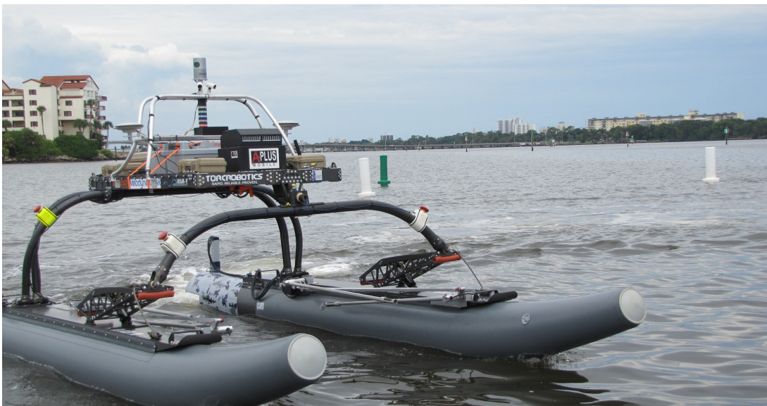
Figure 1: Minion ASV, during a test in the Halifax river in Daytona Beach, FL.
