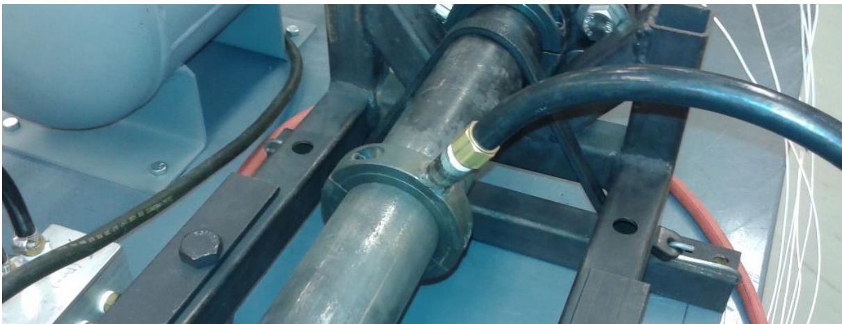
Figure 17 JICF Clamp on Air Manifold in the aft position
