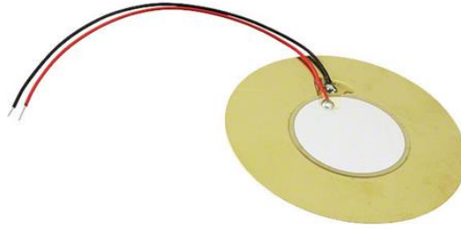
Figure 3.5 Piezo ceramic disc used as driver for SJA.
