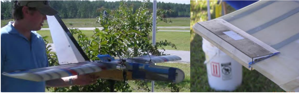
Figure 2.4 Modified dragon eye test bed aircraft (left) and SJA array installed at wing tip (right) (Johnson et al., 2011).
