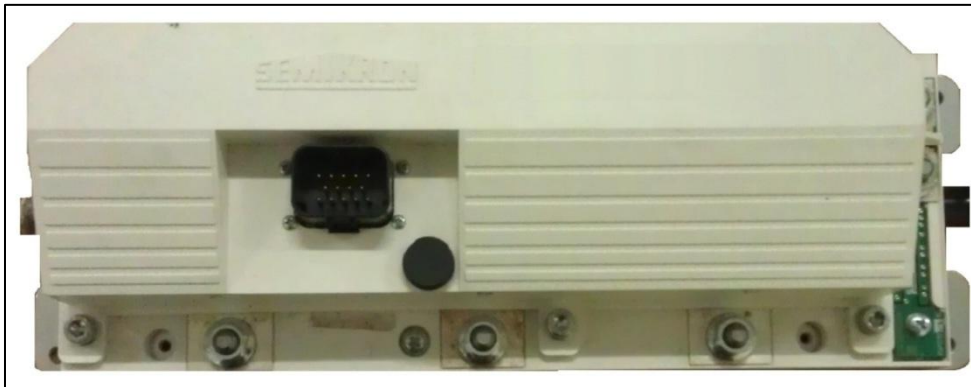
Figure 13: Motor Control Unit
