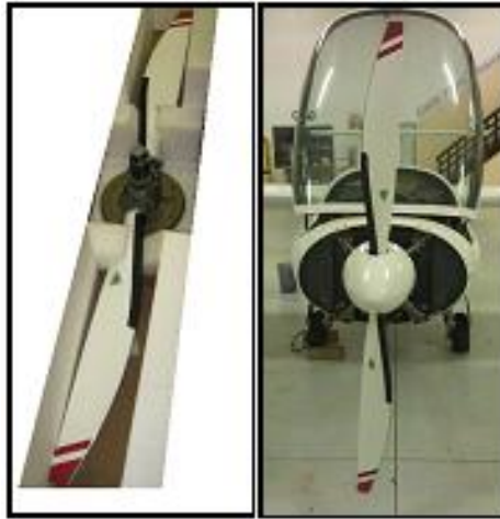
Figure 18: Experimental MT-Propeller for the Eco-Eagle
