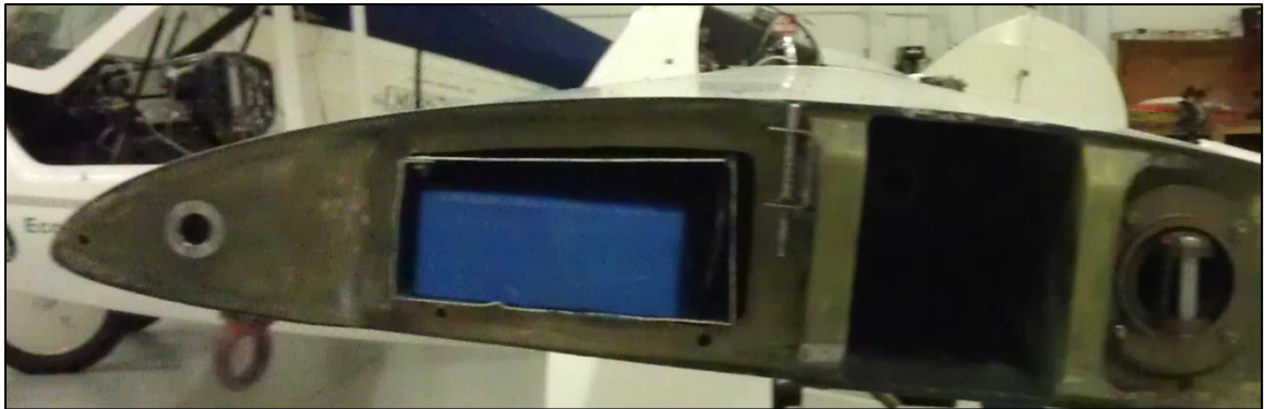
Figure 27: Wing Cutout for Battery Tray
