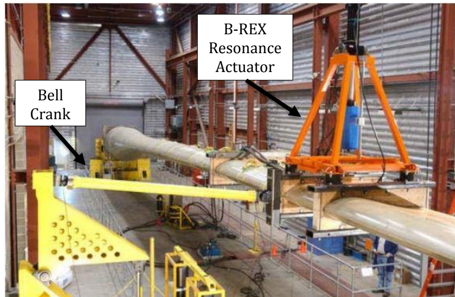
Figure 2.4: B-REX Test Set-up
