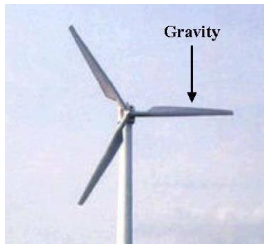
Figure 1.8: Gravity Load Affecting Wind Turbine Blade [15]
