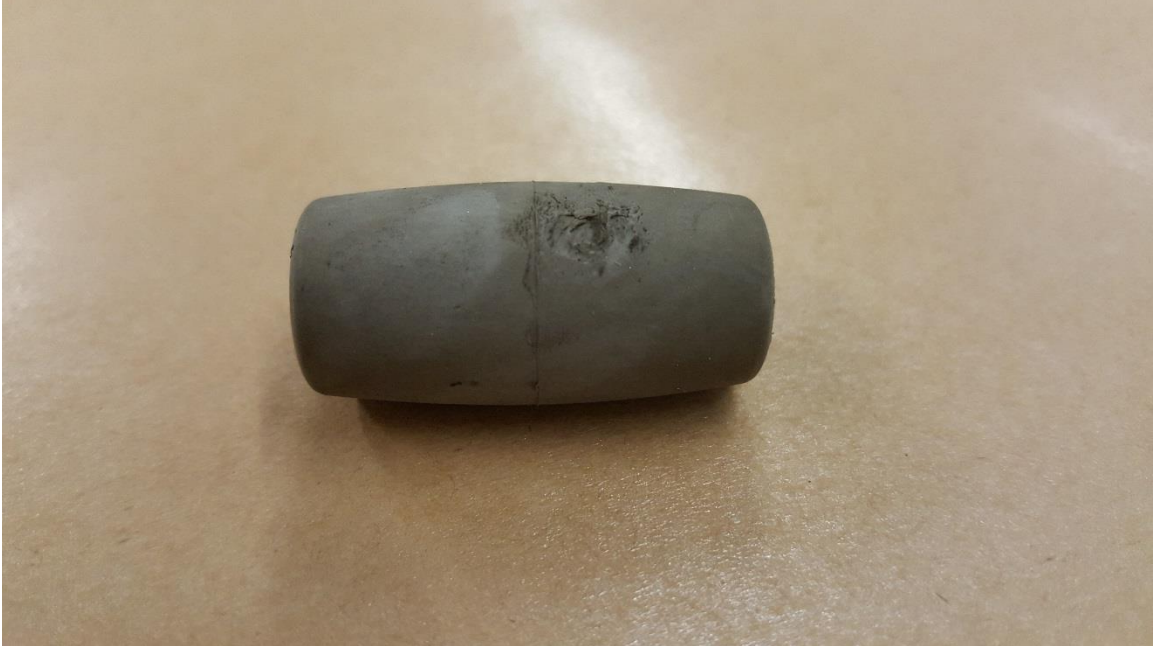
Figure 4.3 Wearing of Roller
