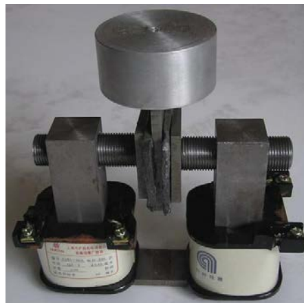
Figure 1.15 MRE experimental setup (Deng, Gong & Wang, 2006)
