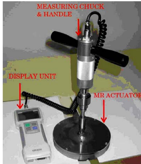
Figure 1.9 MR fluid joystick for haptic force applications (Liu, Li, Kosasih, and Zhang, 2006)
