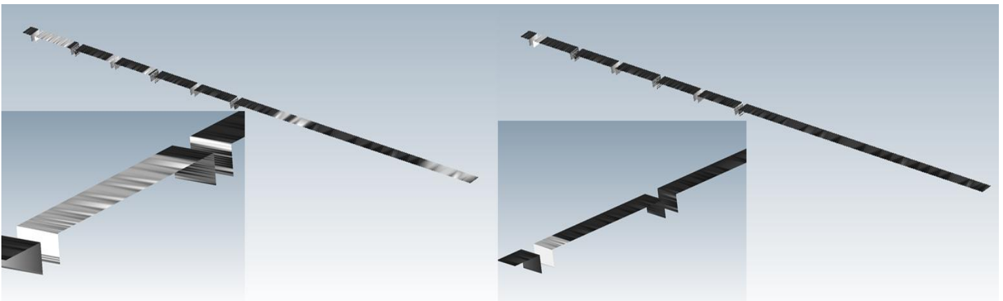
FIGURE 96: ICE ACCUMULATION (FREESTREAM TEMPERATURES OF -20C LEFT, -10 RIGHT)
