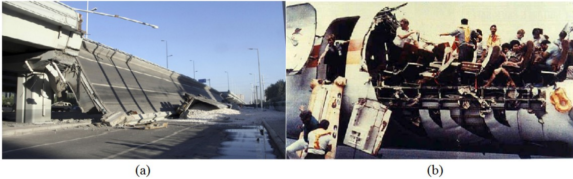
Figure 1. Catastrophic accidents due to structural failures (a) the decompression of Aloha Airlines Flight 243 fuselage [1] (b) a collapsed bridge in China due to poorly controlled construction process [2]
