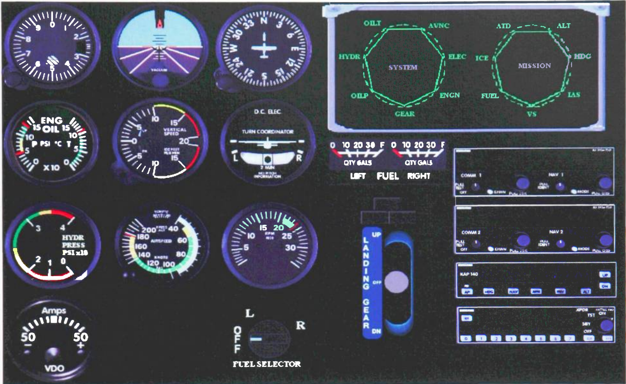
Figure 3 – “Instrument Panel View” with Mission Status Graphics Display
