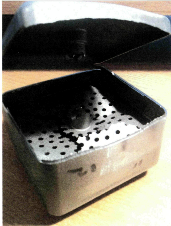
Figure 3-4. The baffle and center post failure.
