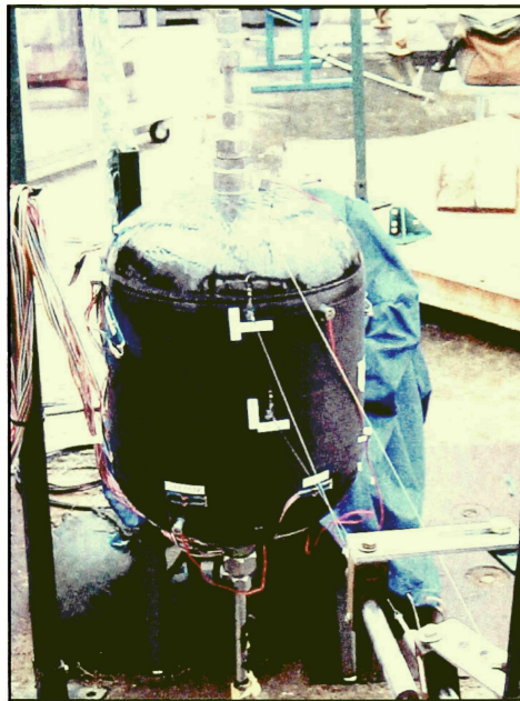
Figure 3: Representative COPV used in burst pressure testing
