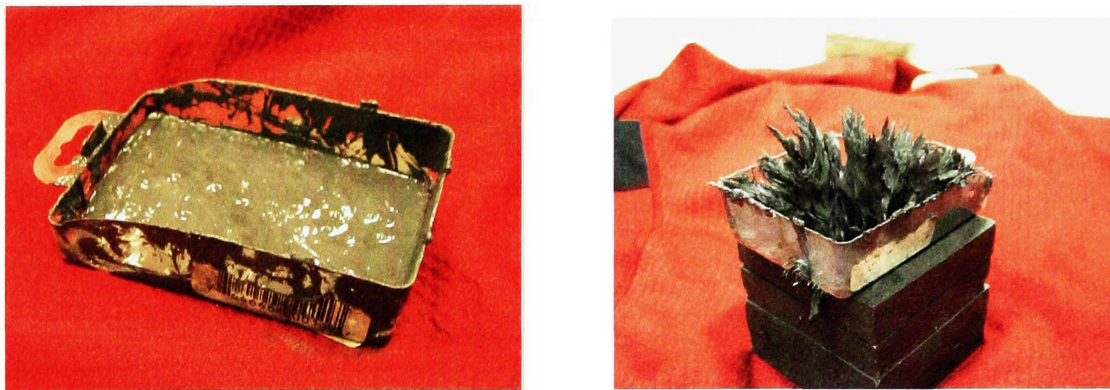
Figure 11. MR Fluid Without a Magnetic field (left) and With a Magnetic field (right) 15 .
