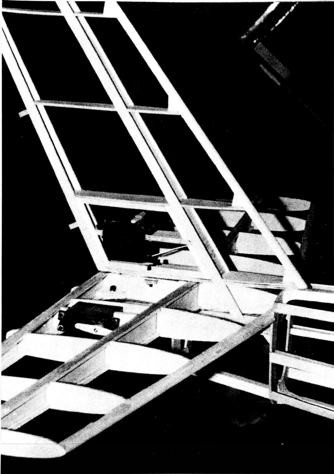
Figure B.12: Vertical and Horizontal Stabilizers Mounted to Aft Fuselage Tailcone
