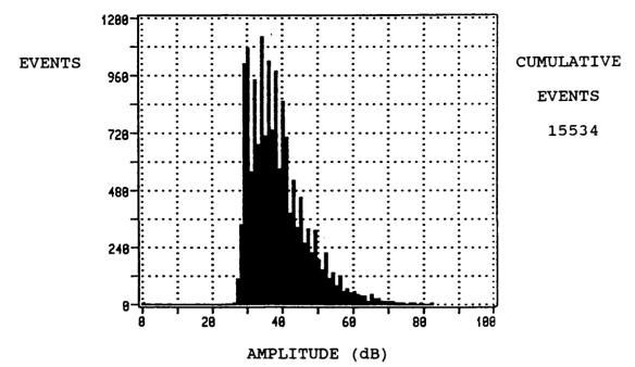
Figure 3. Events Versus Amplitude (dB) Plot for Load Applied Parallel to the Fiber Direction.
