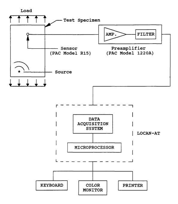
Figure 6. A Typical Test Setup and Configuration.
