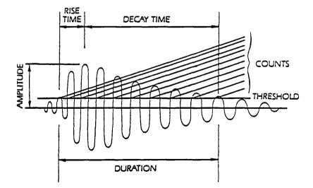
Figure 2. Event Waveform Characteristics [5].
