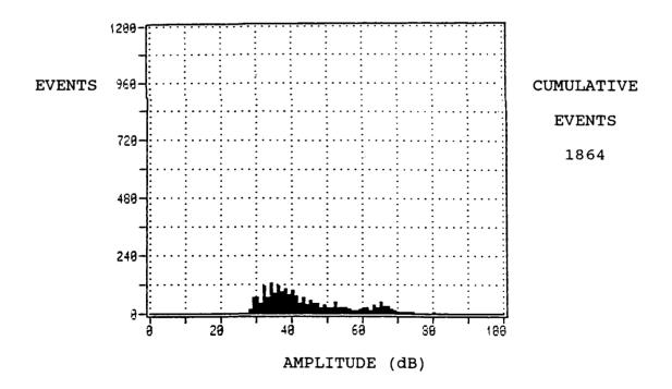
Figure 4. Events Versus Amplitude (dB) Plot for Load Applied Perpendicular to the Fiber Direction.
