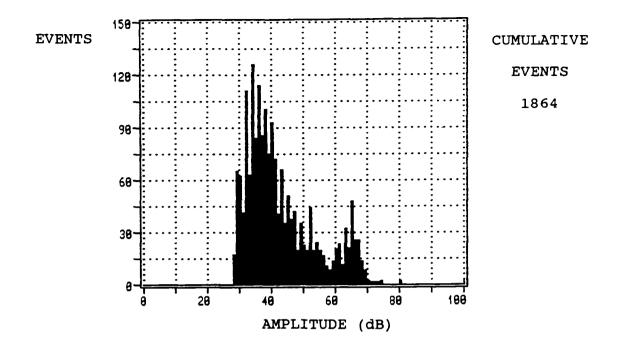
Figure 5. Events Versus Amplitude (dB) Plot of Figure 4 Enlarged.
