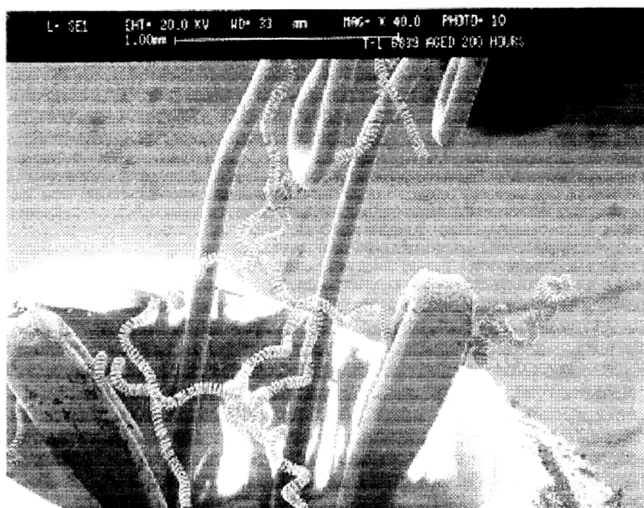
Figure 60. 36839 lamp at 50X, age 200 hours
