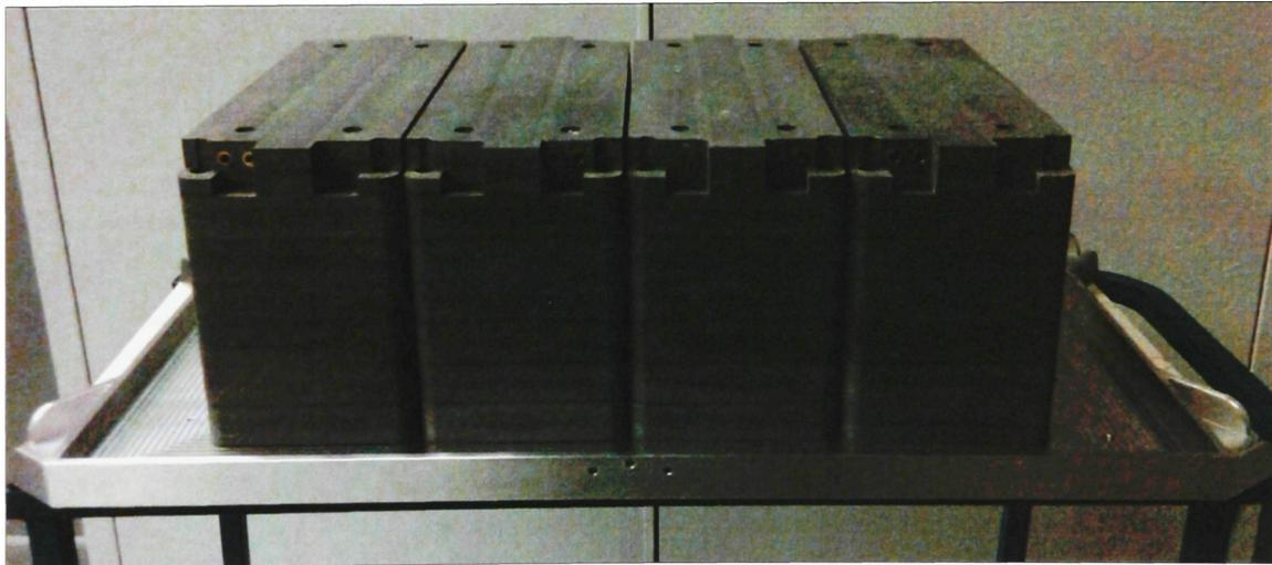
Figure 41: Finished Structural Cold Plate with A123® 25S2P Module Mock Ups
