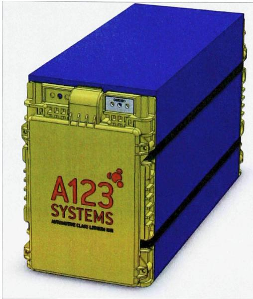
Figure 7: SolidWorks® Model of 25S2P Module
