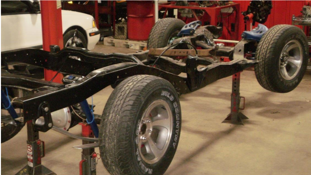
Figure 5.3 S-10 Frame with Painted Brake Component, NERSAT Automotive Technology Program, April 10, 2018
