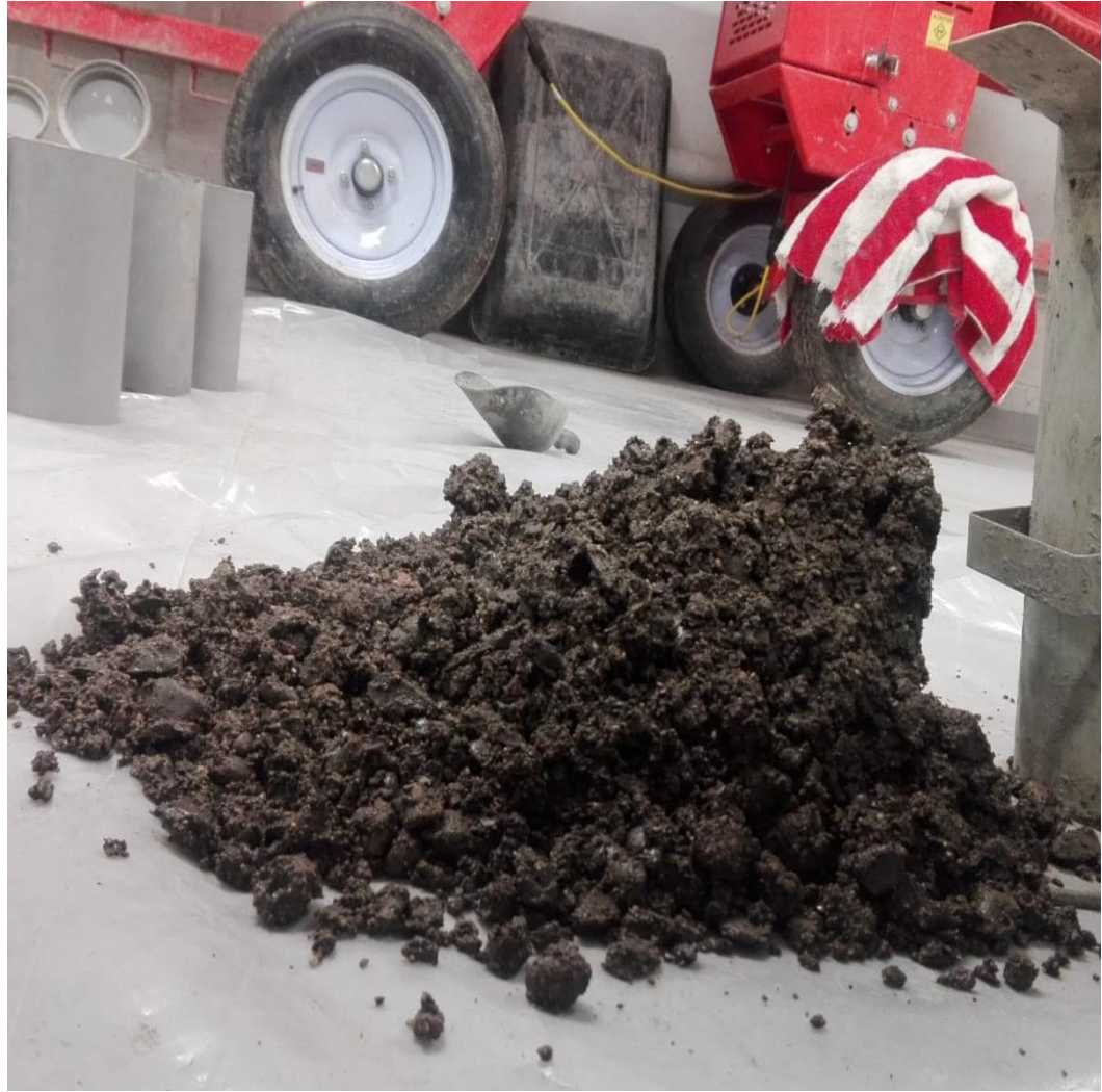
Figure 20: Slump cone test of CLSM mix produced using wood ash
