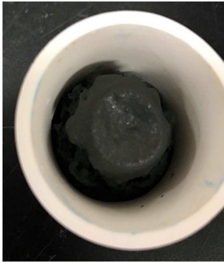
Figure 23 : Lab produced wood ash cement clinker before incinerating
