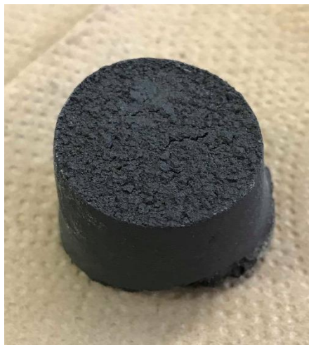
Figure 23 : Lab produced wood ash cement clinker before incinerating
