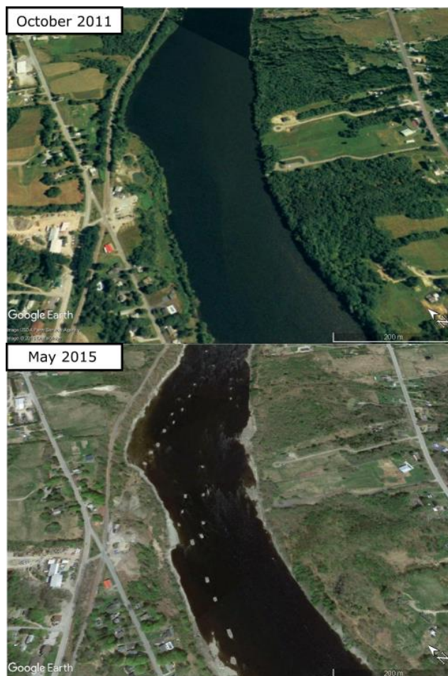
Figure 3.3 – Orthoimagery of the Penobscot River (~53 rkm) Before and After the 2013 Veazie Dam Removal
