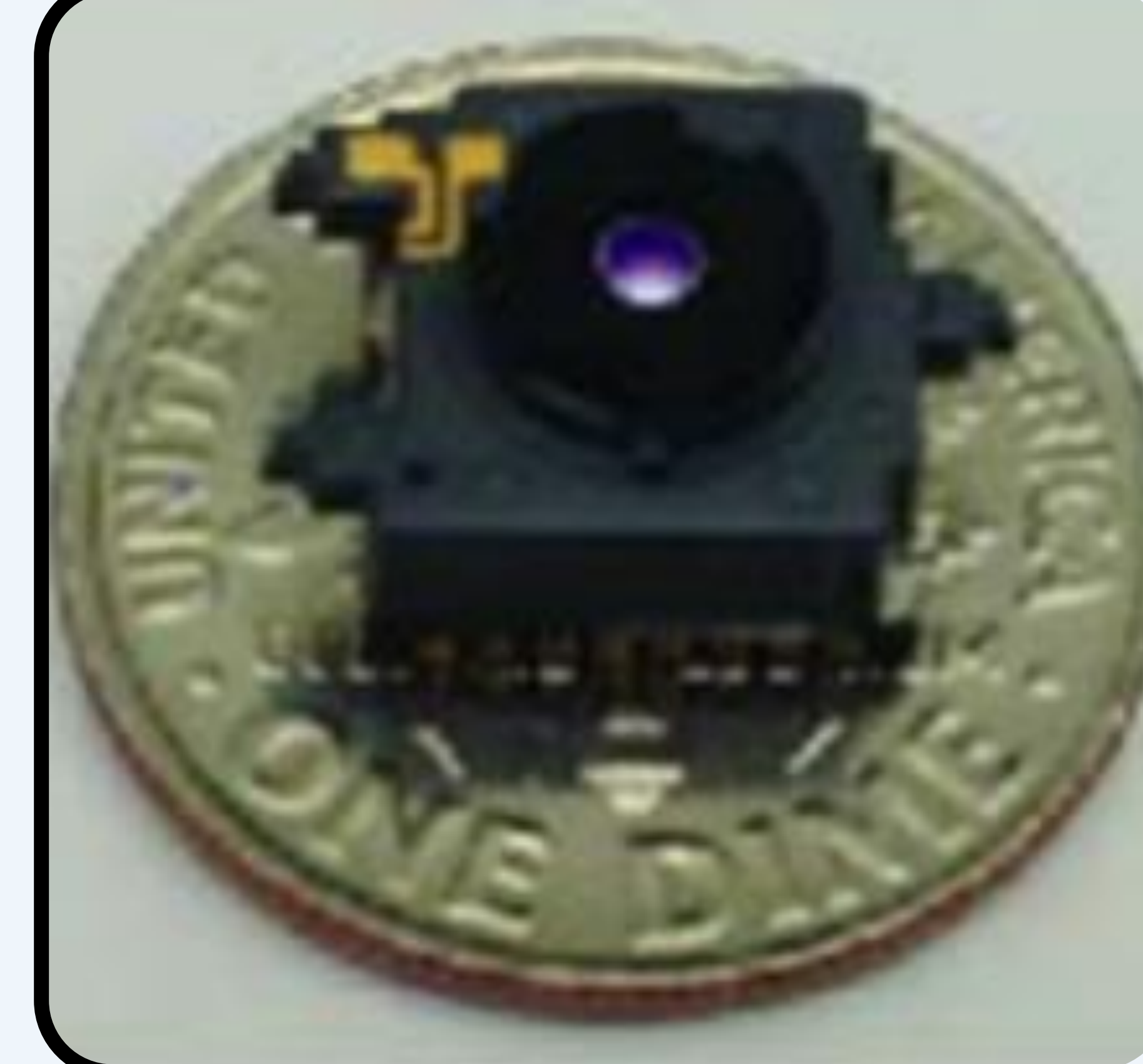
FLIR Lepton with a dime for size comparison.
