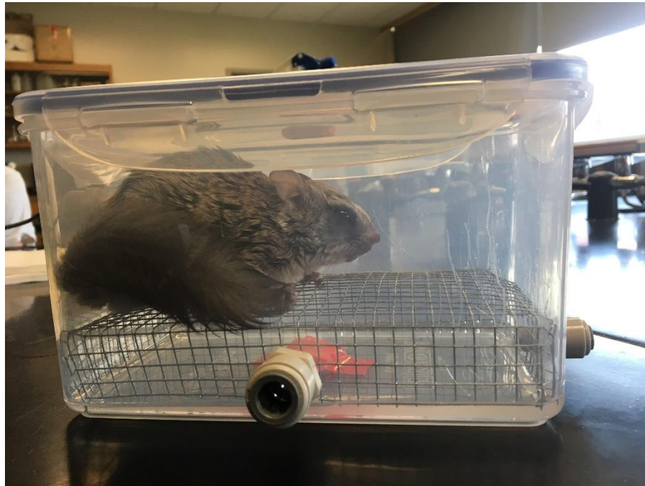
Figure 3: Glaucomys volans in metabolic chamber used for respirometry experiments.
