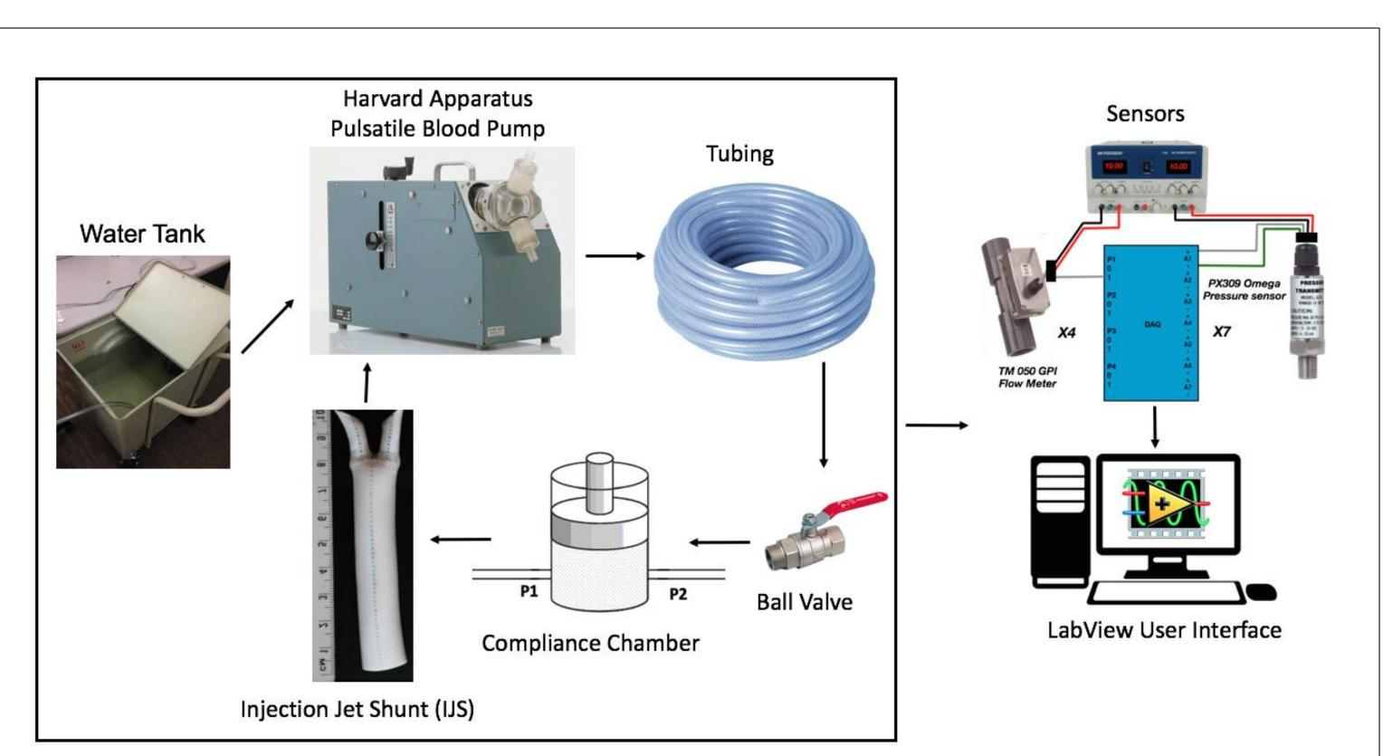
Figure 7. Schematic of flow loop showing individual parts.
