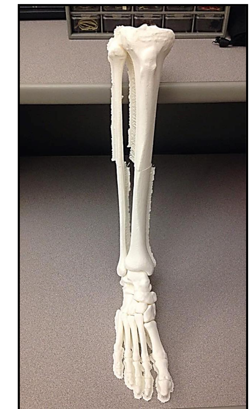
Figure 10. Foot and tibia have been 3D printed with a scaling factor of 4
