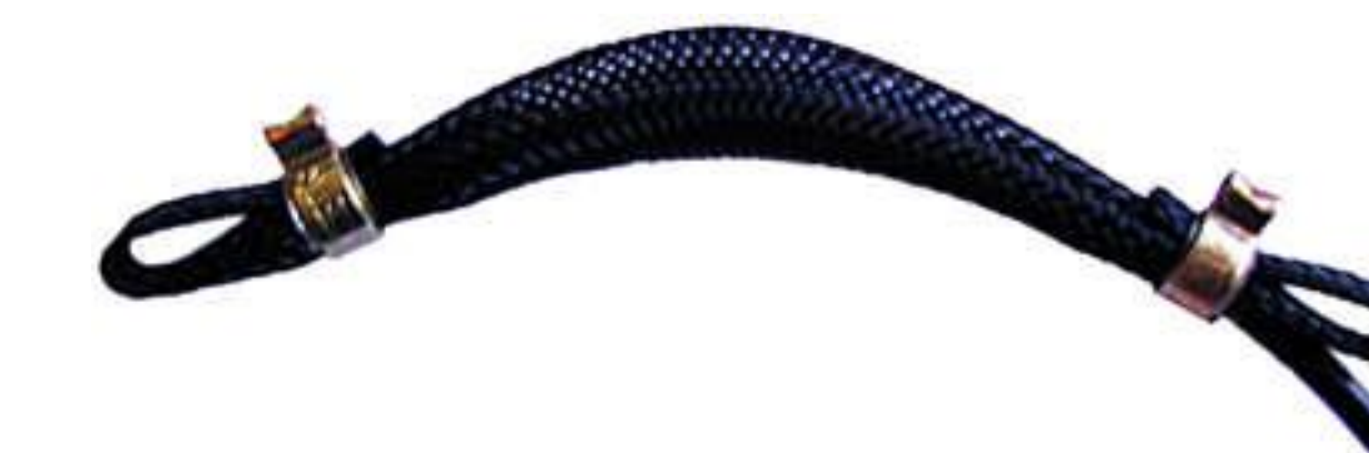
Figure 9. McKibben air muscles have been chosen to replicate the individual force vs. stretch curves. By varying the pressure, the passive muscle force can be adjusted
