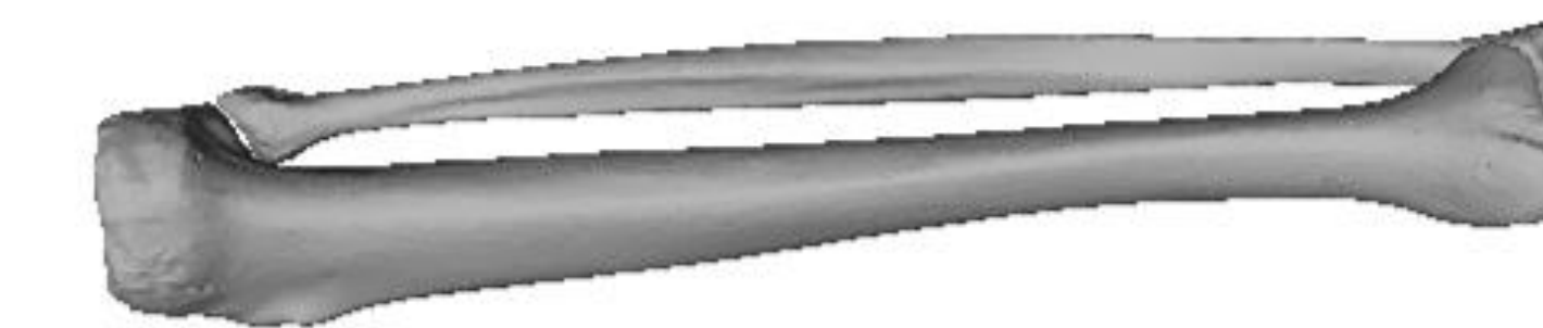
Figure 8. The lower extremities were generated from 3D scans imported to SolidWorks and converted to STL files for 3D printing.
