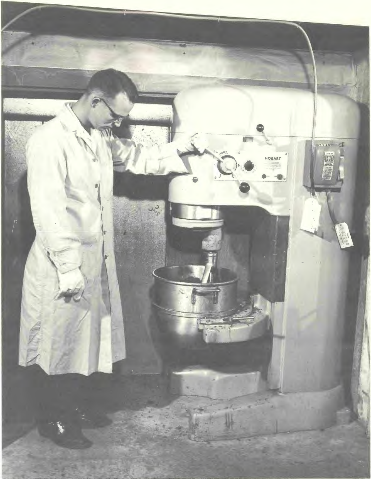
Figure 6 Mixing the Ablative Material
