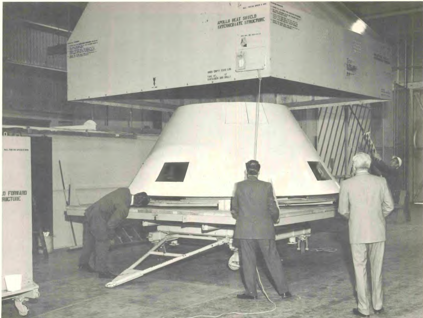
Figure 5 Shipping The Completed Crew Compartment
