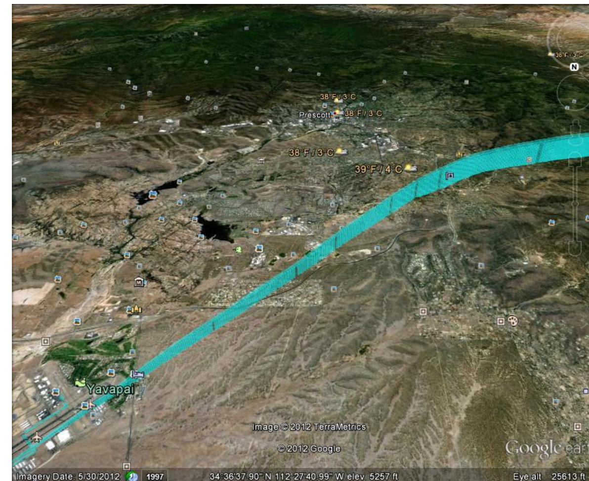
Figure 2 indicates the approach and landing path of an ERAU Prescott training aircraft, using aircraft position data recorded by the G1000 onboard instrumentation system.
